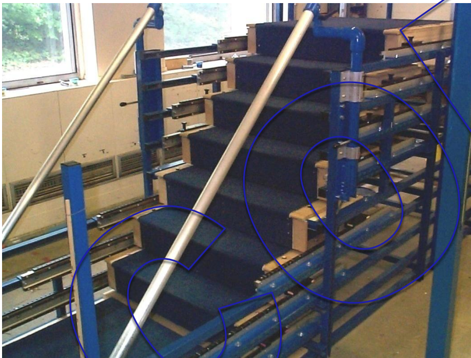
Adjustable steps, designed and used at BRE
